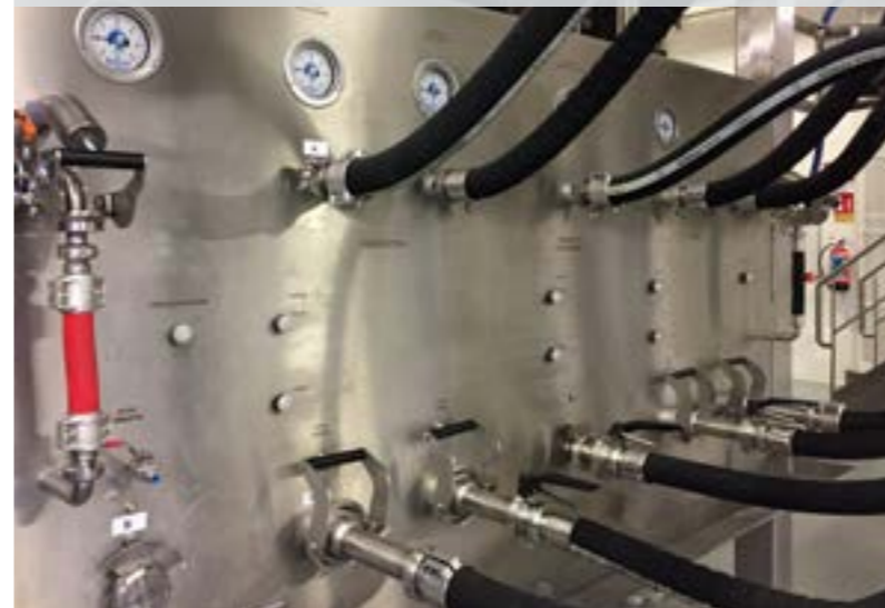
Transfer panel for raw material introduction and sample taking with cleaning in place of hoses and rods
