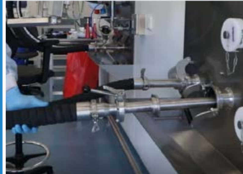
Boclock with handle on the TP side for suction rod (reverse BocLock)
